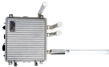
LoRawan outdoor base station
